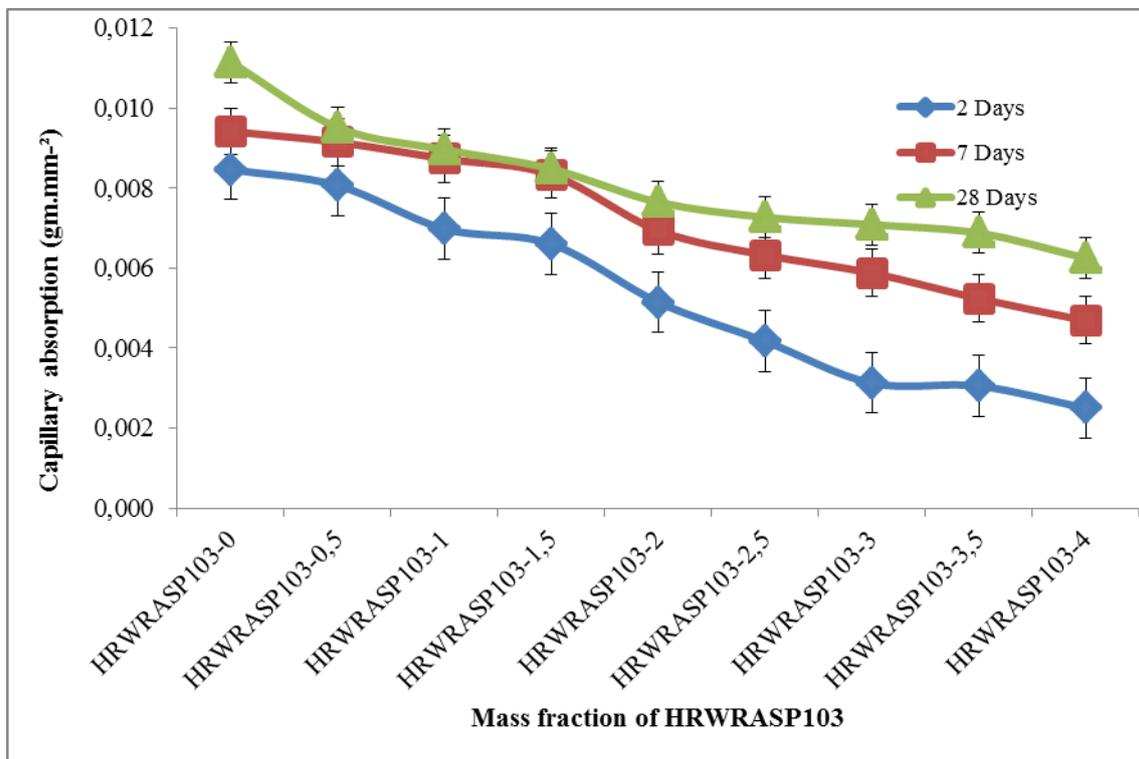
**Figure 11: Variation of the capillary absorption as a function of the mass fractions of HRWRASP103**
