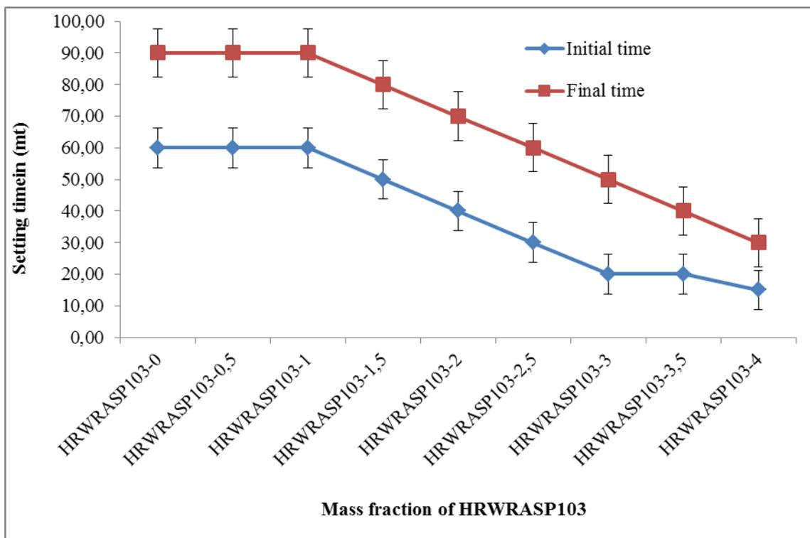
**Figure 9: Variation of the setting time as a function of the mass fraction of HRWRASP103**
