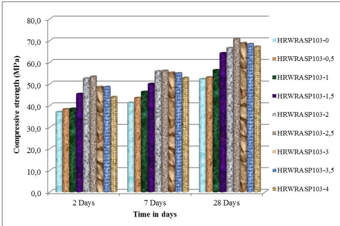
**Figure 13: Variation of compressive strength as a function of time in days**
