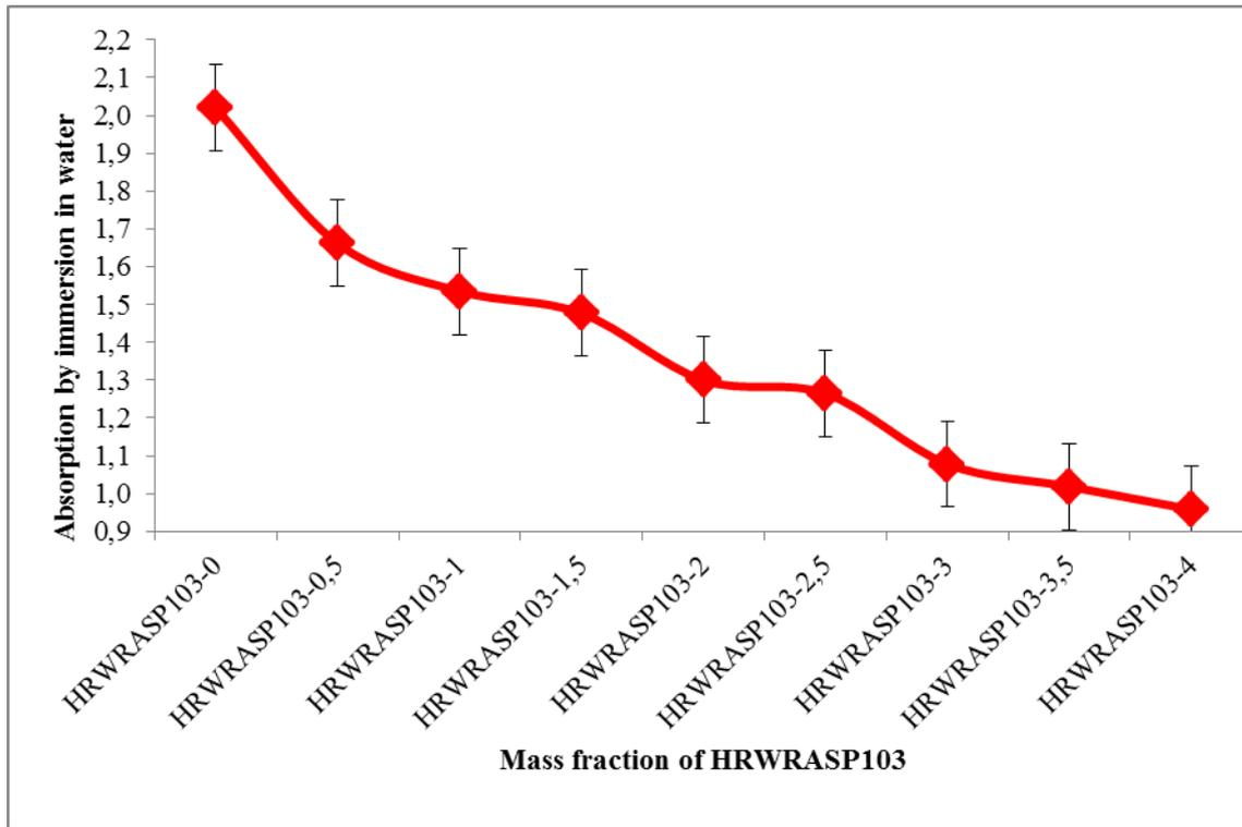
**Figure 12: Variation of the absorption by immersion in water as a function of the mass fractions of HRWRASP103**
