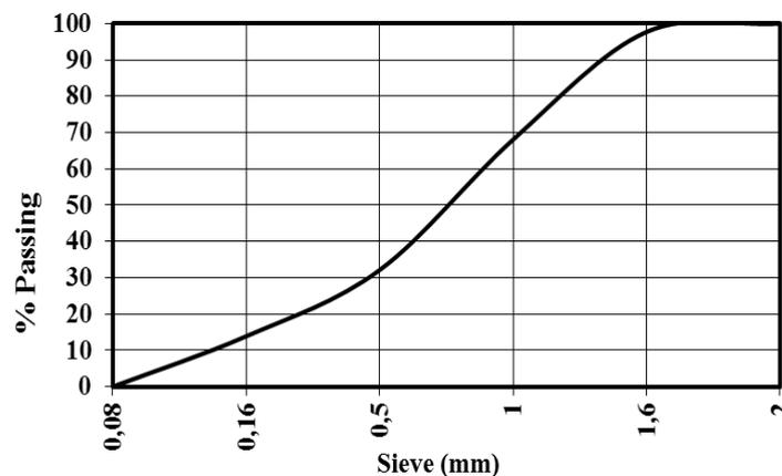
**Figure 4: Curve granulometric of sand**
