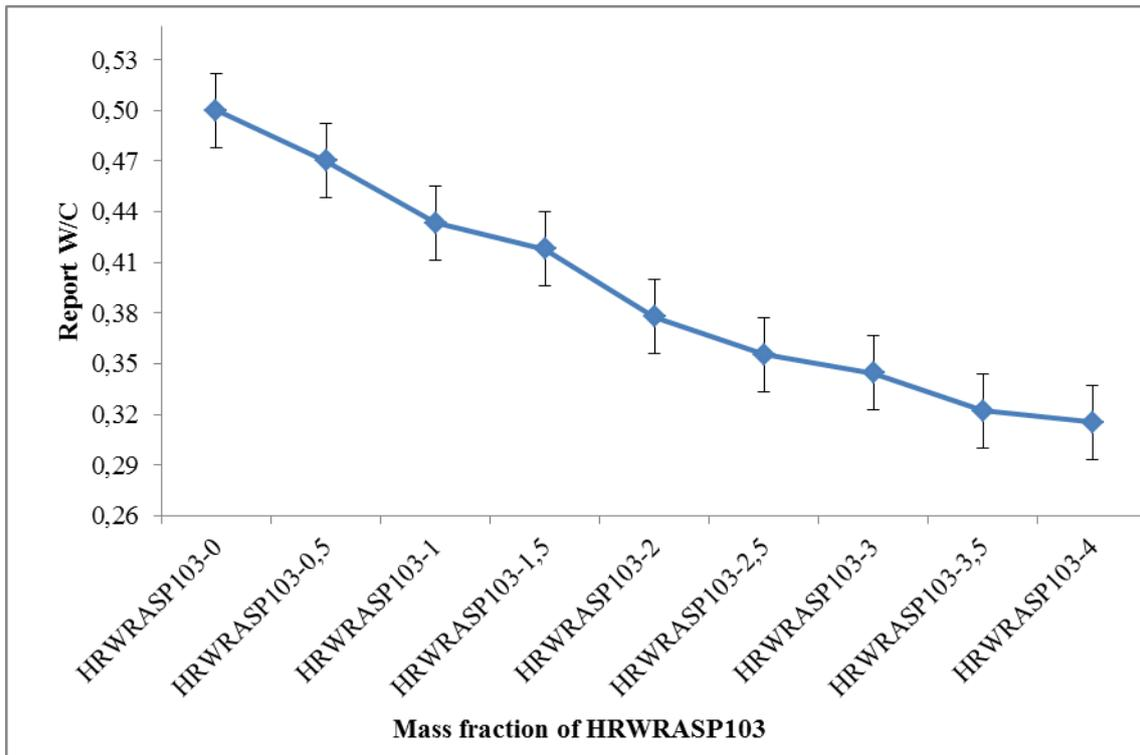
Figure 8: Report of W/C as a function of the mass fraction of HRWRASP103
