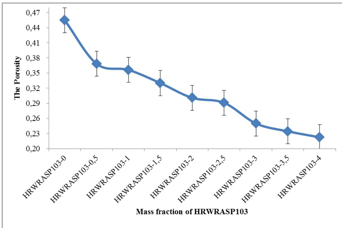
**Figure 10: Variation of the porosity as a function of the mass fractions of HRWRASP103**
